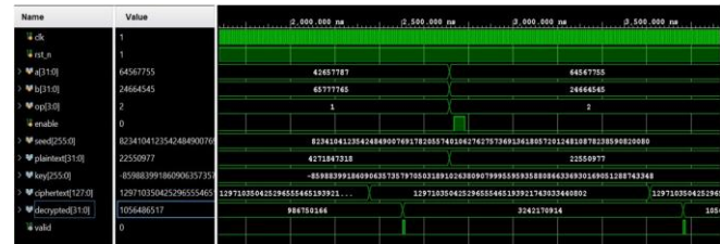
Fig. 8. Integrated PQC-secured RISC-V simulation; decrypted output does not yet match the plaintext.
